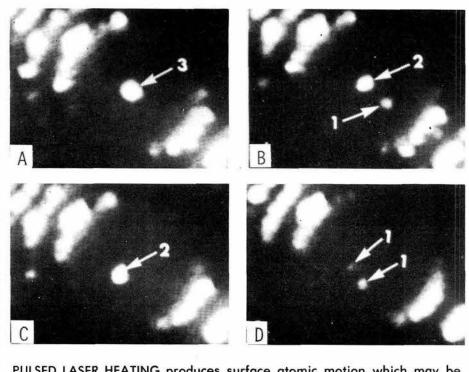
PULSED LASER HEATING produces surface atomic motion which may be observed directly through a field ion microscope. Photo A shows a cluster of three atoms. One of the three has broken away in Photo B. Additional laser pulse heating causes the single atom to break away from the surface (Photo C). The cluster of two atoms breaks apart in Photo D.
